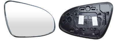
6. COVER, OUTER MIRROR GLASS WITH HEATER (RH)
